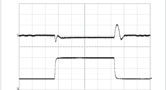
Output Load Transient Response, Default PID/NLR
