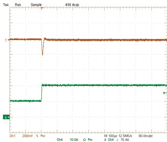
Step Load Transient Response (Vin=5V, Vout=1.2V, Cload=94µF, Iout=6A to 12A) Trace 1=Vout, 200 mV/div, Trace 4=Iout, 10A/div.
