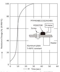
Relation between resistance change and time after POSISTOR PTFM04BE222Q2N34BS is installed on the part heated at a constant temperature of 90°C (3mm thick alminum sheet) is shown in the figure above.
