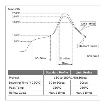
(3) There may be a risk of unexpected failures (tombstone, insufficient solder-wetting, etc.) in the mounting process, caused by the mounting conditions. Please make sure that this product is correctly mounted under specified mounting conditions.
