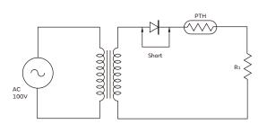
(4) Short - Circuit Test of Electrolytic Capacitor
