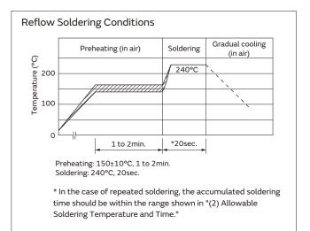
(4) There may be a risk of unexpected failures (tombstone, insufficient solder-wetting, etc.) in the mounting process, caused by the mounting conditions. Please make sure that this product is correctly mounted under the specified mounting conditions.
