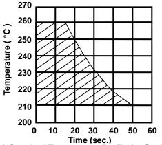
(4) Standard Temperature Profile for Soldering
