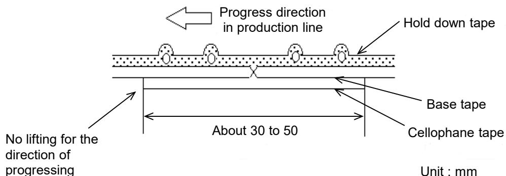
b) When hold down tape is spliced
