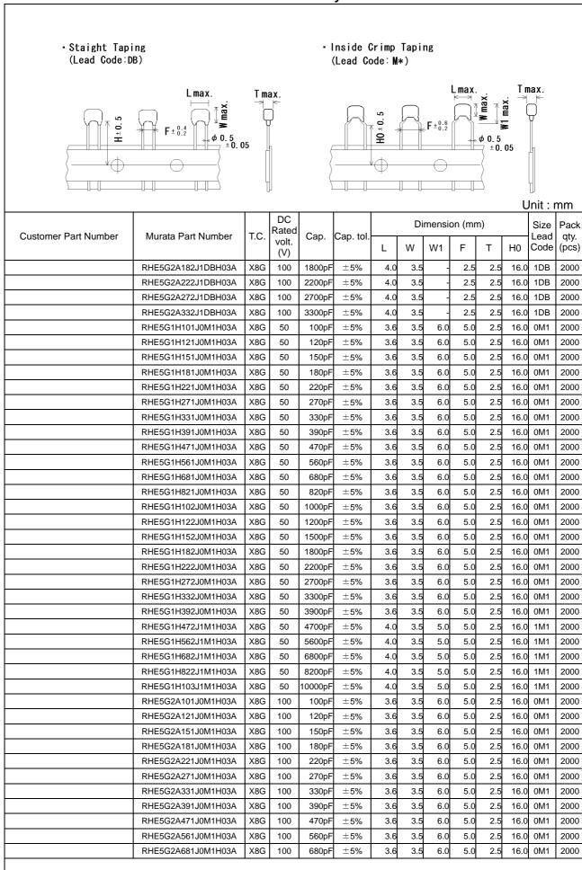
Inside Crimp Taping (Lead Code: M\*)
