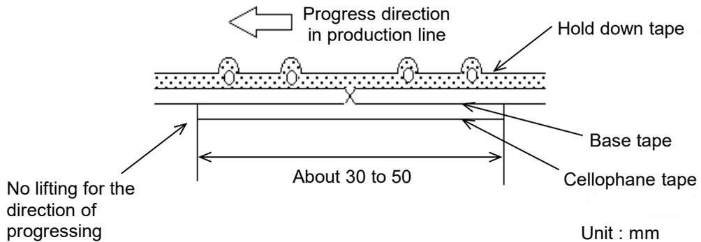
b) When hold down tape is spliced
