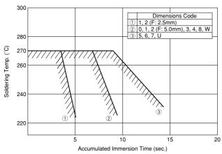
Perform soldering within tolerance range (shaded portion).
