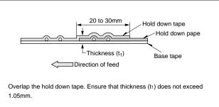
• If both hold down tape and base tape have been cut :
