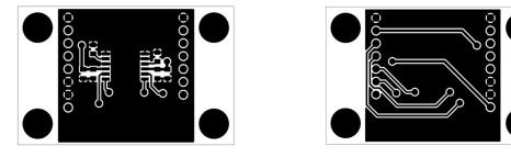
Figure 2. TOP (left) and BOTTOM (right) layout of SCA3300 PCB (aspect ratio not 1:1).
