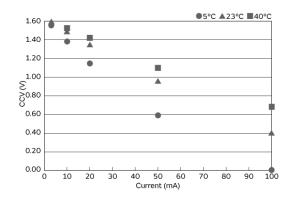
Discharge Characteristics (Load/Temperature)
