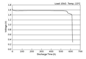
Discharge Characteristics (Load/Temperature)
