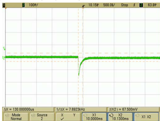
Step Load Transient Response (Slew=1A / \mu Sec., Vin=48V., Clod=0, Iout=22.5A to 15A)
