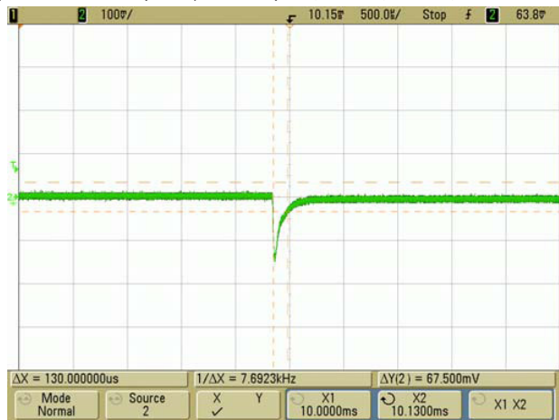
Step Load Transient Response (Slew=1A / \mu Sec., Vin=48V., Cload=0, Iout=22.5A to 15A)
