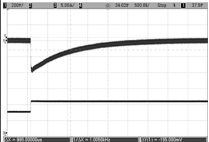
Step Load Transient Response (Vin = 48V, Vout = nom, Cload = 1µF || 10µF, Iout = 50 to 75 to 50% of full load, Ta = +25°C) Ch1 = Vout, Ch2 = Iout.
