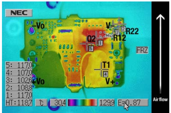
Thermal image with hot spot at full load with 85 °C ambient; air is flowing at 400LFM. Air if flowing across the converter from +V to -V at 48V input. Identifiable and recommended value to be verified in application. (Q2, max temp=120 °C/IPC9592 guidelines)
