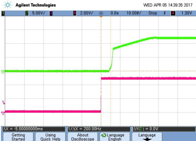
On/Off Enable Delay (Vin = 12V Vout = nom Iload = 0A Load = 200μF CH2: Vout; CH4: Enable; Ta = +25°C)
