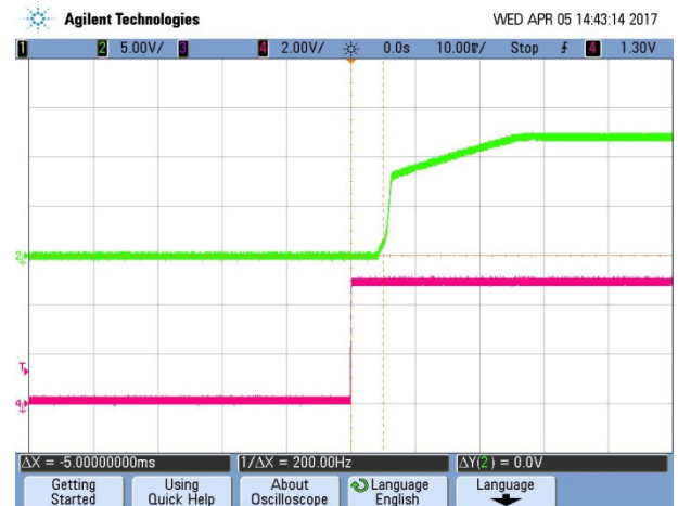
On/Off Enable Delay (Vin = 12V Vout = nom Iload = 0A Load = 4700μF CH2: Vout; CH4: Enable; Ta = +25°C)
