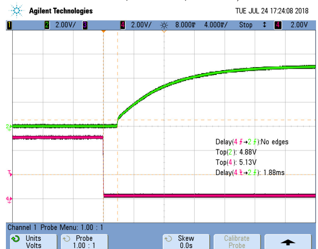
On/Off Enable Delay (Vin = 12V Vout= nom load =0A Load=4700μF CH2: Vout; CH4: Enable; Ta=+25°C)
