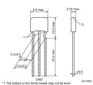
\*2 There may be a hole on the top of ferrite beads, which causes no characteristics deterioration.
