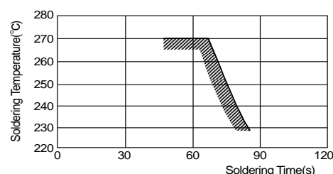
[Allowable Reflow Soldering Temperature and Time]
