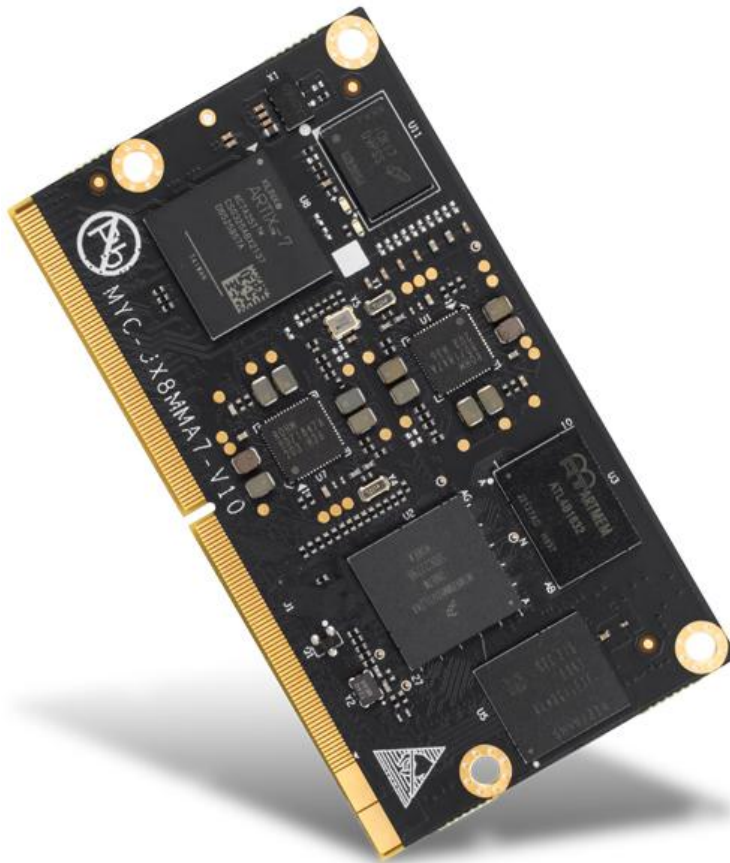
Figure 1-1 MYC-JX8MMA7 CPU Module
