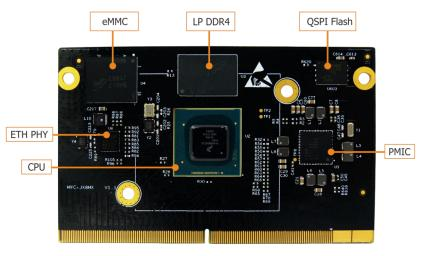
Figure 1-2 MYC-JX8MX CPU Module
