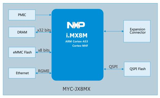
Figure 1-6 MYC-JX8MX CPU Module Function Block Diagram
