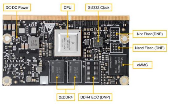
Figure 1-5 MYC-J1028X CPU Module Top-view
