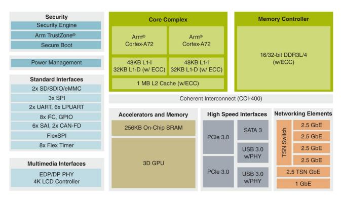
Figure 1-4 Layerscape LS1028A System Block Diagram
