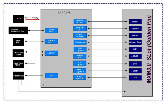
Figure 1-7 MYC-J1028X CPU Module Function Block Diagram
