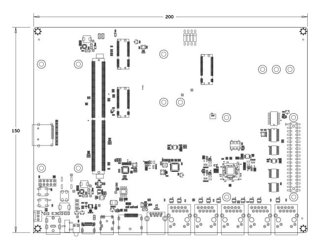
Figure 1-10 MYD-J1028X Base Board Dimensions Chart (Unit: MM)
