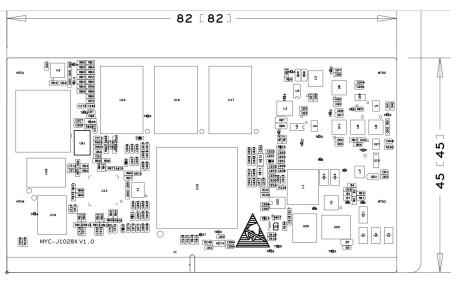
Figure 1-9 MYC-J1028X Dimensions Chart (Unit: MM)
