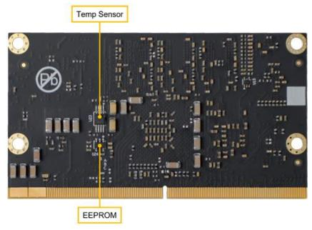
Figure 1-6 MYC-J1028X CPU Module Bottom-view
