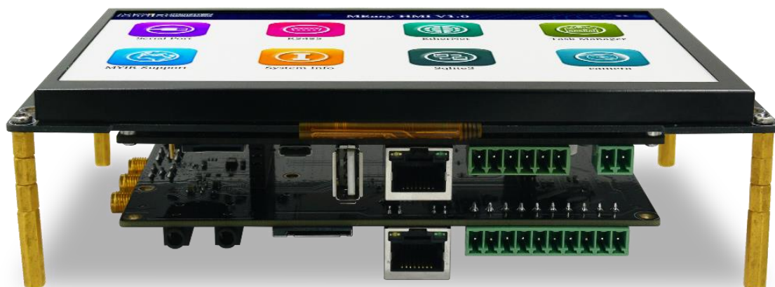
Figure 1-6 MYD-Y6ULX-CHMI Display Panel + MYB-Y6ULX-HMI-4GEXP IO Board
