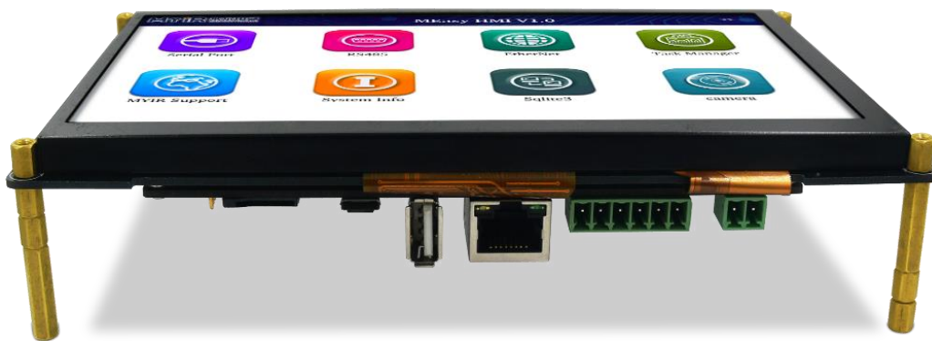
Figure 1-5 MYD-Y6ULX-CHMI Display Panel
