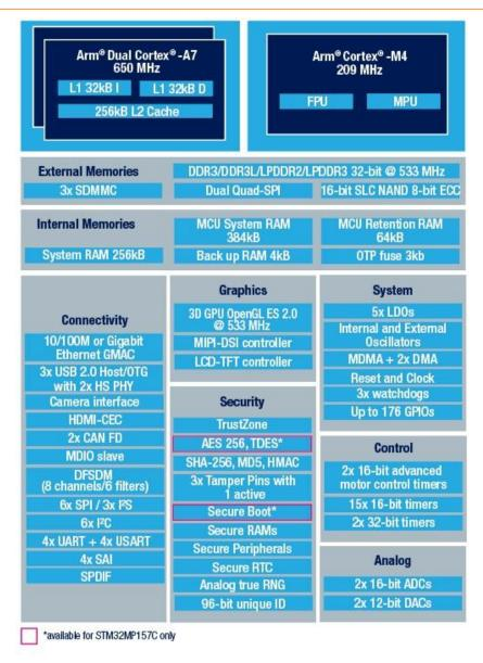
Figure 1-5 STM32MP157 Block Diagram
