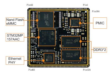
Figure 1-6 MYC-YA157C CPU Module
