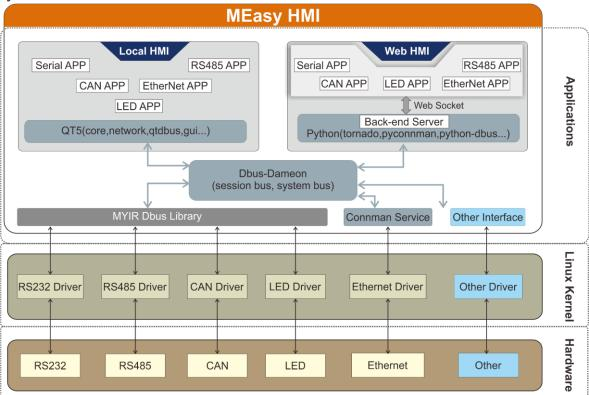
Figure 1-12 MEasy-HMI System Structure
