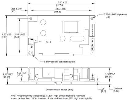
Note: Recommended standoff size is: 375<sup>°</sup> high and all mounting hardware should be less than .28" in diameter. A standoff less than .375<sup>°</sup> high is acceptable when a thin insulator, 0.4mm thick (polyester, fish paper or equivalent UL rated 94V-2 minimum) is placed between the XL160 and the mounting chassis (refer to applicable UL standard for clearance requirements).
