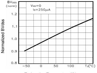
TJ-Junction Temperature(℃) Figure 9 BV<sub>DSS</sub> vs Junction Temperature
