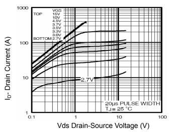
**Figure 1 Output Characteristics**
