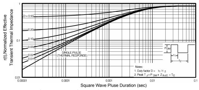
**Figure 11 Normalized Maximum Transient Thermal Impedance**
