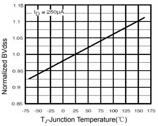
Figure 9 BV<sub>DSS</sub> vs Junction Temperature
