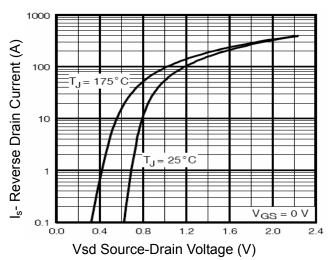
Figure 6 Source- Drain Diode Forward
