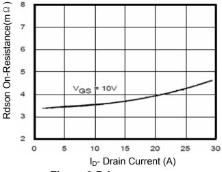
Figure 3 Rdson- Drain Current
