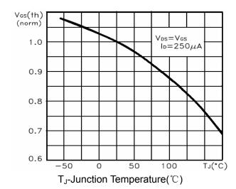
Figure 10 V<sub>GS(th)</sub> vs Junction Temperature
