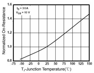
Figure 4 Rdson-JunctionTemperature
