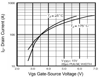
**Figure 2 Transfer Characteristics**
