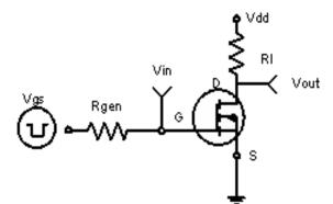
Figure 1:Switching Test Circuit
