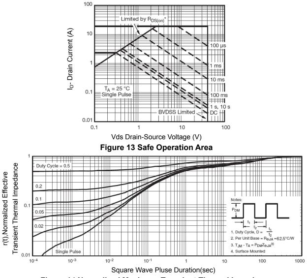
Figure 14 Normalized Maximum Transient Thermal Impedance
