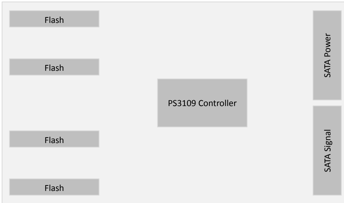
Figure 2: mSATA Controller Block Diagram
