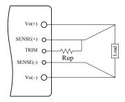
Figure 16 Circuit to Increase Output Voltage
