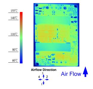
Figure 11. Thermal Image for Airflow Direction 3 (24.3A output, 55°C ambient, 200 LFM, typical Vin, open frame, unit soldered onto a fixture board.)
