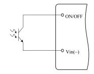
Figure 12. Opto Coupler Enable Circuit
