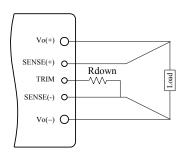
Figure 15 Circuit to Decrease Output Voltage
