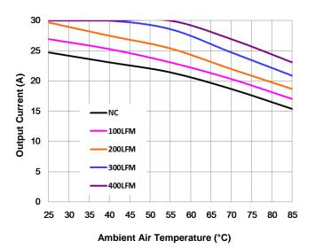
Figure 8. Current Derating Curve for Airflow Direction 1 (Ref. Figure. 9 for Airflow Direction; typical Vin, open frame, unit soldered onto a fixture board.)
