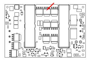
Figure 17. Temperature Monitoring Location
