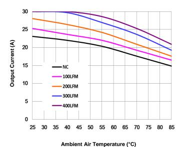
Figure 10. Current Derating Curve for Airflow Direction 3 (Ref. Figure.11 for Airflow Direction; typical Vin, open frame, unit soldered onto a fixture board.)
