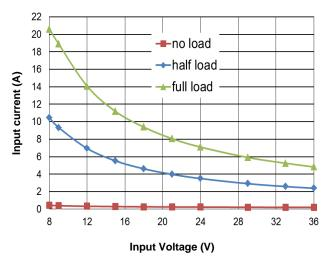
Figure 3. Input Characteristics
