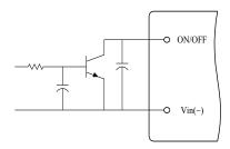
Figure 13. Open Collector Enable Circuit
