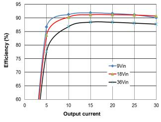
Figure 1. Efficiency vs. Load Current (25°C)
