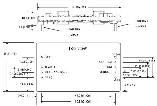
Figure 18. Open Frame Converter
