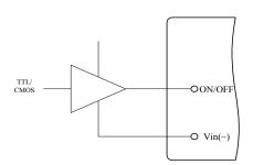
Figure 14. Direct Logic Drive
