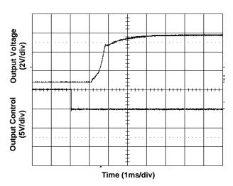
Figure 4. Start-Up from Enable Control (Typical input voltage and full load)
