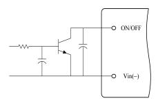
Figure 16. Open Collector Enable Circuit
