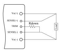
Figure 18. Circuit to Decrease Output Voltage
