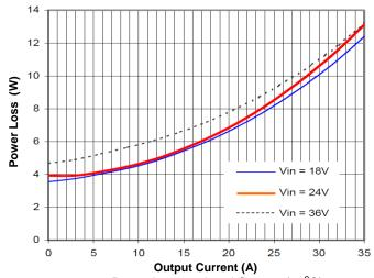
Figure 2. Power Loss vs. Load Current (25°C)
