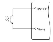
Figure 15. Opto Coupler Enable Circuit
