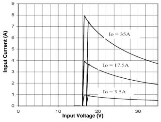
Figure 9. Input Characteristics
