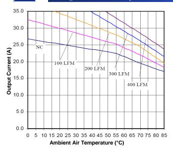
Figure 11. Current Derating Curve for Airflow Direction 3
