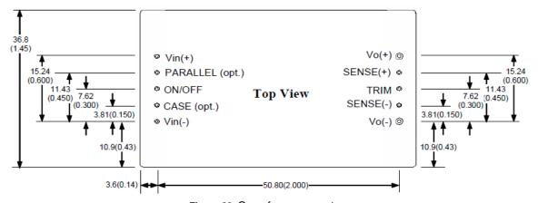
Figure 22. Open frame converter
