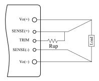
Figure 19. Circuit to Increase Output Voltage
