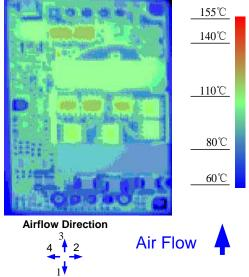
Figure 14. Thermal Image for Airflow Direction 4 (24.8A output, 55°C ambient, 200 LFM, Vin = 24V open frame unit using solder interface)
