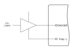
Figure 17. Direct Logic Drive
