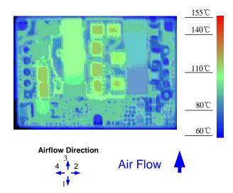
Figure 12. Thermal Image for Airflow Direction 3 (28A output, 55°C ambient, 200 LFM, typical Vin, open frame unit using soldering interface)
