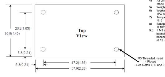
Figure 23. Converter with a baseplate
