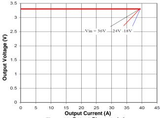
Figure 10. Output Characteristics
