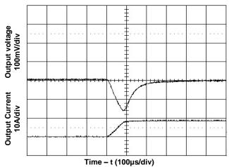
Figure 8. Transient Load Response
