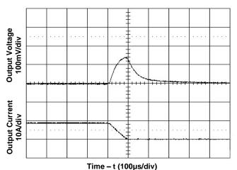
Figure 7. Transient Load Response
