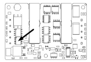
Figure 21. Temperature Monitoring Location
