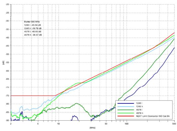
The results of the pairs 4578 seem to be below the limits in the frequency range of 10 to 20 MHz. However, this is a snapshot of an instantaneous signal trace frozen in time. Very low signal levels below 65 dB are susceptible to small changes in the physical arrangement of DUT and fixture. In this sense the limit line is not really violated. Furthermore, in this very low frequency range there is ample headroom to the channel specifications.
