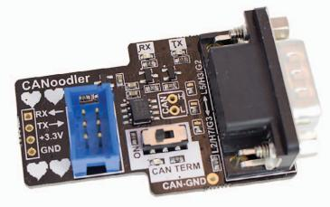
CANoodler is a simple CAN (not CAN-FD) interface, which provides logic-level 3.3V output. It's designed to be used with microcontrollers that have CAN blocks inside them, and in particular uses a pinout present on some ChipWhisperer CW308 (UFO) Target boards.
