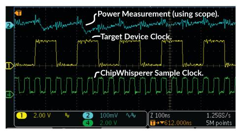
Our ChipWhisperer capture hardware can use a target device clock and apply multiplications and phase shifts to sample at desired point(s) during the clock cycle. This ensures sample points are directly related to the digital clock which generates the signals of interest. The result is many devices can be successfully attacked with 5-100x slower sample clock compared to a regular oscilloscope.
