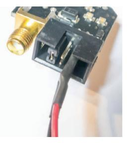
Using a single-ended supply means connecting the -V input to the GND pad. This is done via a jumper mounted as shown on the 6-pin connector on left.
