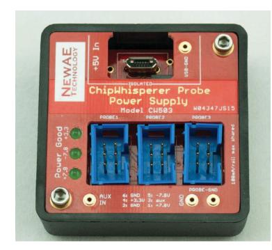
The probe power supply is designed to provide power to the differential probe and low noise amplifier.
