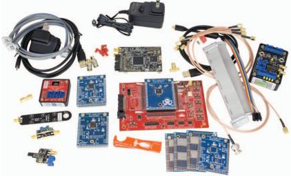
This starter pack extends the Level 1 pack by adding the features needed for working with external targets (besides the included UFO targets). The advanced breakout board can perform level-shifting when you aren't working with 3.3V I/O or need additional breakout.
