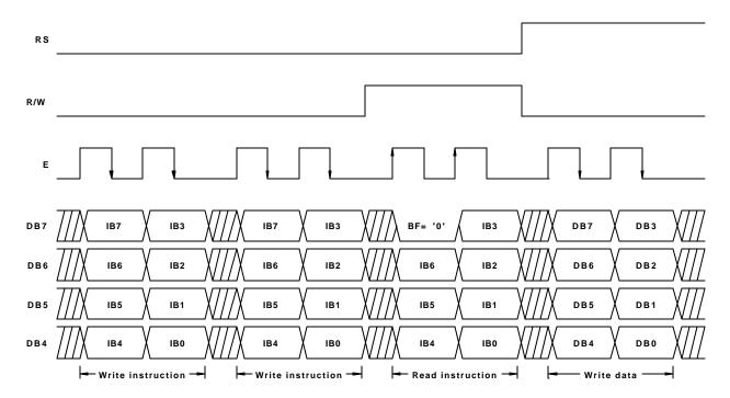
Figure 9. Typical 4-Bit Parallel Interface Sequence Using M68-Type Mode
