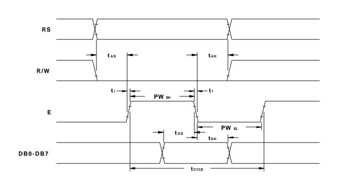
Figure 3. Motorola M68-Type Parallel Interface Write Cycle Timing
