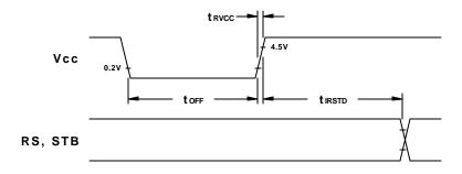
Figure 1. Power-up Internal Reset Timing
