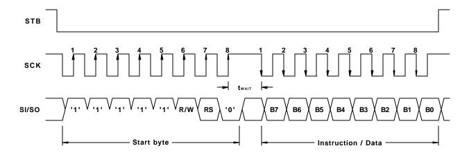
Figure 12. Typical Synchronous Serial Interface Read Cycle
