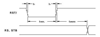
Figure 2. External Reset Timing
