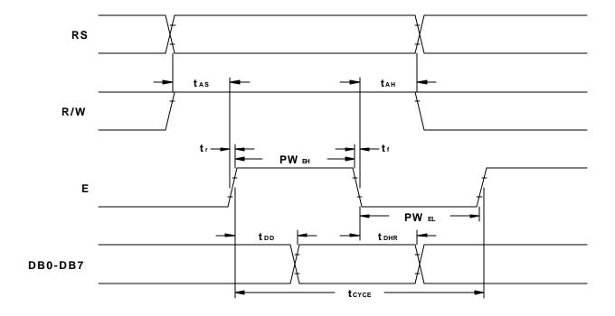
**Figure 4.** Motorola M68-Type Parallel Interface Read Cycle Timing
