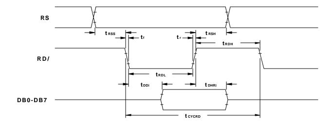
Figure 6. Intel I80-Type Parallel Interface Read Cycle Timing
