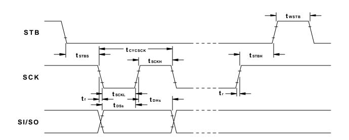
**Figure 7.** Synchronous Serial Interface Write Cycle Timing
