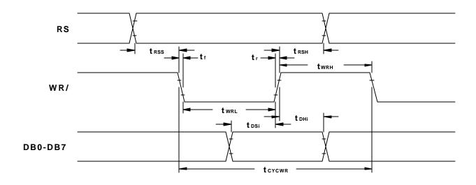
Figure 5. Intel I80-Type Parallel Interface Write Cycle Timing
