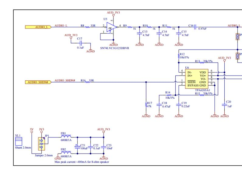
This is a reference schematic from FTDI, which can be used to successfully filter and amplify the audio signals coming from t
