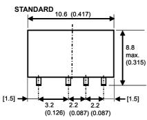
Tolerance of lead pitch is  $\pm 0.15$ mm (0.006inch) Other tolerances  $\pm 0.3$ mm (0.012inch)
