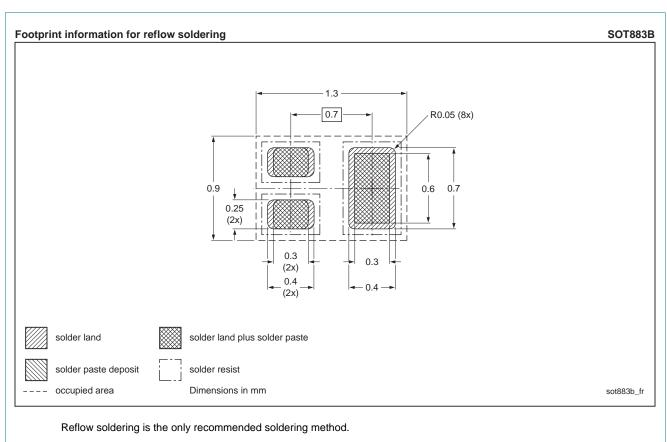
Fig 4. Reflow soldering footprint DFN1006B-3 (SOT883B)
