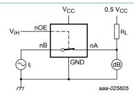
nOE connected to  $V_{CC}$ ;  $f_i$  is biased at  $0.5V_{CC}$ . Adjust  $f_i$  voltage to obtain 0 dBm level at output. Increase f<sub>i</sub> frequency until dB meter reads -3 dB.
