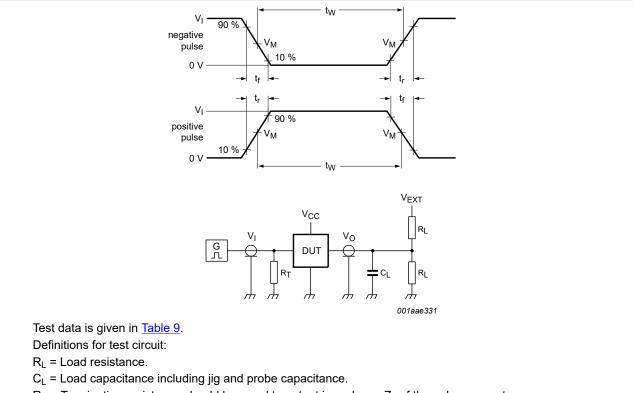
$R_{T}$  = Termination resistance should be equal to output impedance  $Z_{o}$  of the pulse generator.
