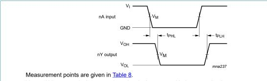
V<sub>OL</sub> and V<sub>OH</sub> are typical output voltage levels that occur with the output load.
