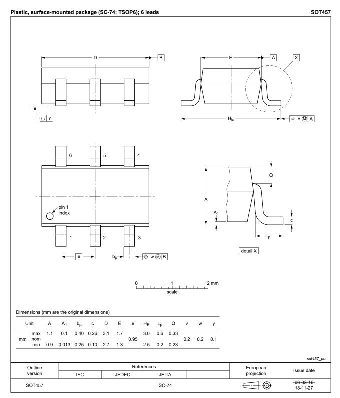
Fig. 8. Package outline SOT457 (SC-74; TSOP6)
