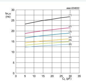
a. HIGH to LOW propagation delay (STCP to Qn)
