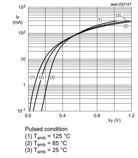
Forward current as a function of forward Fig. 2. voltage; typical values
