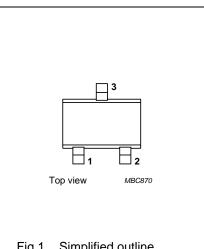
Fig.1 Simplified outline SOT323 and pin configuration.
