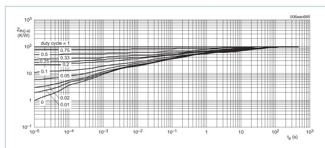
FR4 PCB, single-sided copper, mounting pad for collector 6 cm<sup>2</sup>
