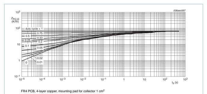
Fig 14. Transient thermal impedance from junction to ambient as a function of pulse duration for SOT1061; typical values
