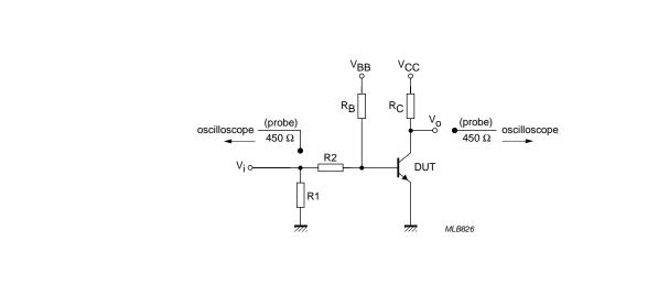
$V_i$  = 0.5 V to 4.2 V; T = 500  $\mu s;$   $t_p$  = 10  $\mu s;$   $t_r$  =  $t_s \leq 3$  ns.
