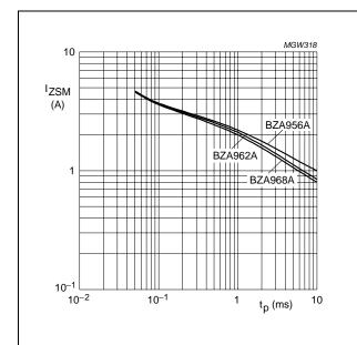
Fig.2 Maximum non-repetitive peak reverse current as a function of pulse time.
