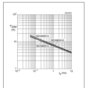
Fig.3 Maximum non-repetitive peak reverse power dissipation as a function of pulse duration (square pulse).
