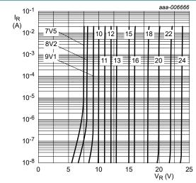
Reverse current as a function of Fig. 9. reverse voltage; typical values (BZT52H-B/C7V5 to BZT52H-B/C24)
