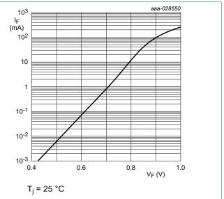
Fig. 2. Forward current as a function of forward voltage; typical values (BZT52H-B/C2V4)
