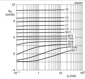
Fig. 7. of working current; typical values
