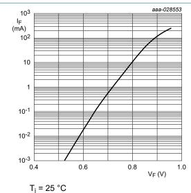
Fig. 5. Forward current as a function of forward voltage; typical values (BZT52H-B/C75)
