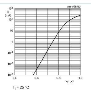
Fig. 4. Forward current as a function of forward voltage; typical values (BZT52H-B/C7V5)
