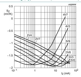
Fig. 6. Temperature coefficient as a function of working current; typical values (BZT52H-B/C2V4 to B/C4V7)
